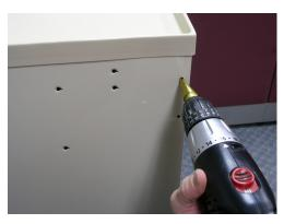
NOTE: A step drill bit is recommended for maintaining the best hole location and quality.
