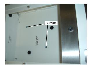
A close-up of one of the SLS PCS threaded holes as seen through the cutout in the shelf frame is shown in the following figure:
