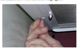
10. Slide the shelf onto the shelf rail. This is done by tilting the shelf into the slots on the shelf rail (as shown in the first figure below) and then pushing down on the shelf until it clicks into place (as shown in the second figure below):
