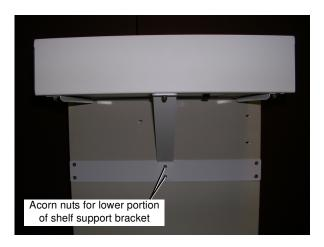
21. Tighten the four shelf support bracket acorn nuts using a 5/16-in. nut driver. Then tighten all four flat-head screws using a P3 Phillips head screwdriver to secure the lower support bracket to the side of the cart.
