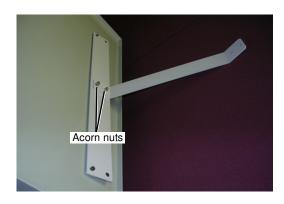
14. Remove the two acorn nuts, shown in the following figure, from the threaded studs on the bottom of the shelf opposite the shelf rail. Set them aside for use in step 20 of the installation procedure.
