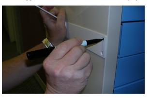
NOTE: If the Blue Bell top shelf support rail is installed use a 6-inch level aligned with the holes of the lower support bracket to determine the location of the mounting holes. Mark the locations on the cart with a permanent marker.
