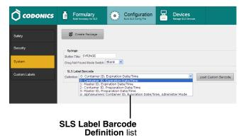
3. Modify other configuration settings as needed, create the configuration package, and deploy the package to 500i devices. For more information about these tasks, refer to the SLS Administration Tool User's Manual.
