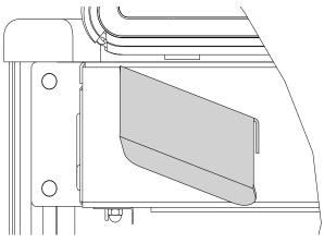
3. Press the holster onto the 500i shelf and apply pressure for 30 seconds to one full minute.
